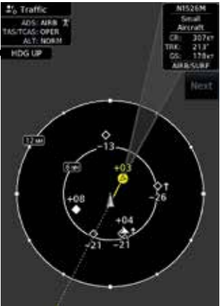
Garmin traffic system alerting provides both visual and spoken audio advisories to help helicopter pilots maintain safe separation from other aircraft in busy airspace.
