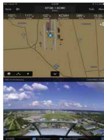
Wireless connectivity lets you stream live video from the VIRB series action cameras onto your Garmin Pilot enabled device or G3X™ cockpit display.
