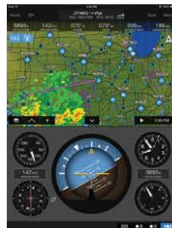
In addition to ADS-B weather and traffic, you can view 3-D synthetic vision and backup AHRS attitude reference provided by the GDL 51/52 series portable ADS-B receivers.
