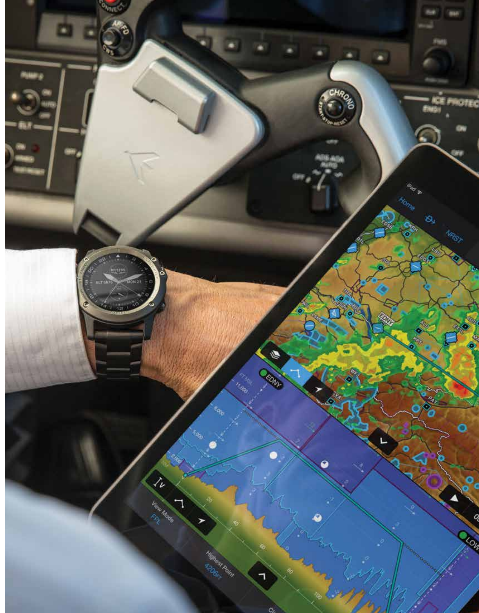
In addition to ADS-B weather and traffic, you can view 3-D synthetic vision and backup AHRS attitude reference provided by the GDL 51/52 series portable ADS-B receivers.
