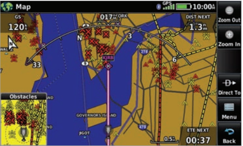
For low-flying helicopters and patrol aircraft, Garmin WireAware™ wire-strike avoidance technology offers added protection against powerline incidents.
