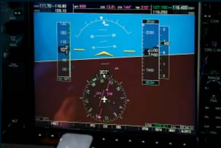
The Garmin G1000's Primary Flight Display with attitude, heading and altitude info
