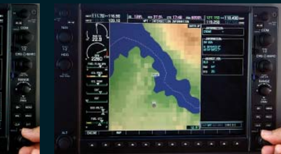
The Garmin G1000's Multifunction Display with intersection information
