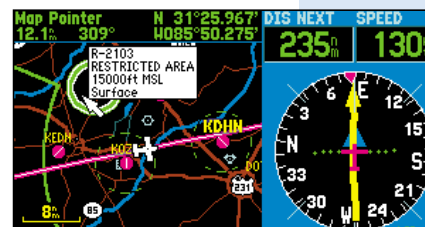
SUA data revealed on map page (screen shown in night mode)
