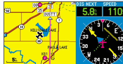
"vector to final" on HSI, moving map split screen
