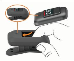
To remove the device from the belt clip, pull the flexible clip material away from the device.
