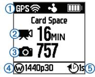
Displays the sensor status and remaining battery capacity. Includes ANT+° sensors, Bluetooth°, Wi-Fi°, and GPS.
