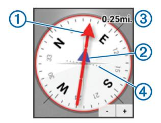
The course pointer ① indicates your relationship to the course line leading to the destination. The course deviation indicator (CDI) ② provides the indication of drift (right or left) from the course. The scale ③ refers to the distance between dots ④ on the course deviation indicator, which tell you how far off course you are.
