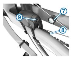
**6** Place the spoke in the groove of the plastic piece, and tighten it slightly.
