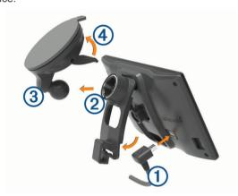
2 Press the mount ② onto the suction cup ③ until it snaps into place.
