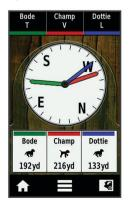
You can use the dog tracking compass to view the direction and distance to your dog. The dog tracking compass also shows the dog's status, such as running or on point (*Dog Status Icons*,
