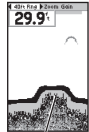
Structure is soft, probably a mud pile
