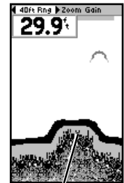
Structure is soft, probably a mud pile
