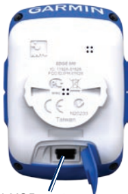
Mini-USB port under weather cap
