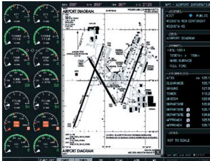
The top photo shows the G1000 MFD in the King Air in the reversionary mode with primary flight information combined with engine instruments and other data. This mode is used after the failure of a PFD display. The other photo above of the MFD shows an airport diagram along with frequencies and other information. On the MFD photo below is a display of precipitation from the onboard Garmin weather radar that is part of the conversion package.
