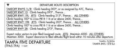
Figure 1. Example Aircraft Type-specific Departure Route Description
