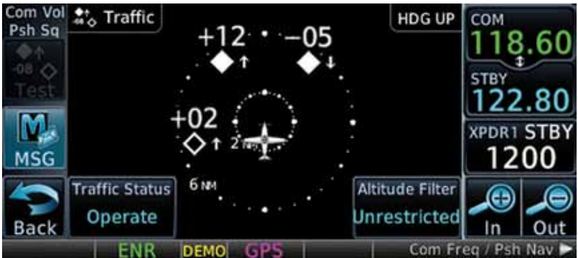
GTS series traffic alerts can be displayed on Garmin’s GTN 650/750 and 430W/530W series avionics.
