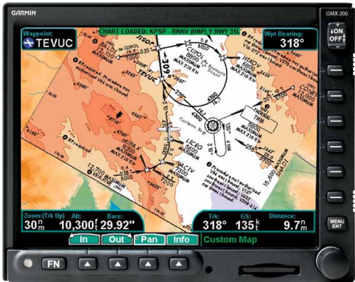
Optional ChartView™: Electronic display of Jeppesen® approach plates is enabled through Garmin's ChartView™ option (subscription required). Instrument approaches and airport surface diagrams can be viewed with the aircraft position overlaid on the GMX 200 display. Based on the flight plan, the GMX 200 will automatically load the approach charts for the destination airport. Standard Instrument Arrival and Departure procedures (STARs and DPs) are also provided.
