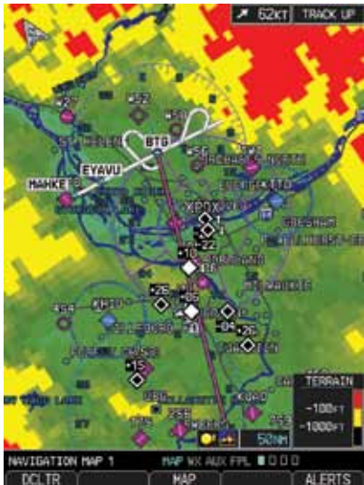
Integration of traffic, terrain and obstacle alerting on a Garmin moving-map display gives pilots a comprehensive picture of potential flight path conflicts.
