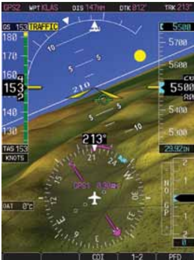
With Garmin’s SVT-capable flight displays, traffic can be depicted in a 3-D format. As targets get closer, the symbols get larger.
